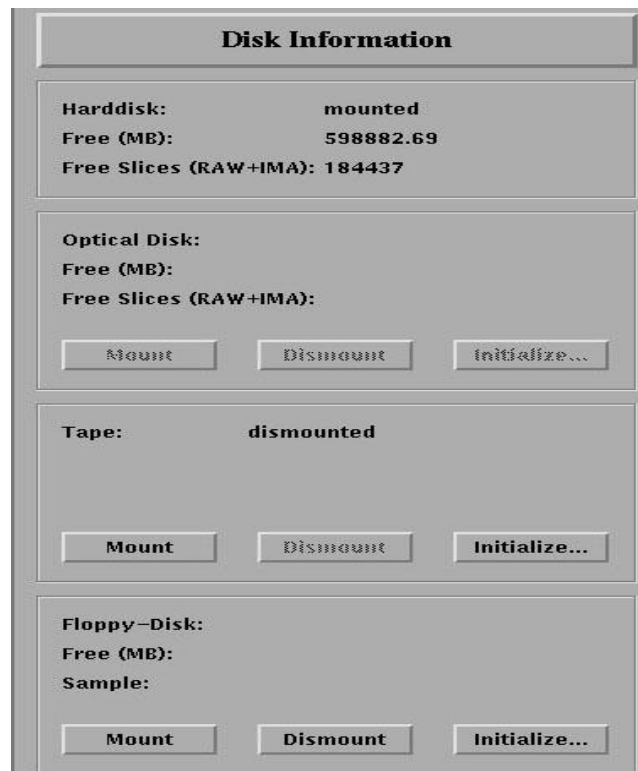
Figure 6: Disk Information section of uct backup tool window, where one can mount, dismount or initialize a tape.
