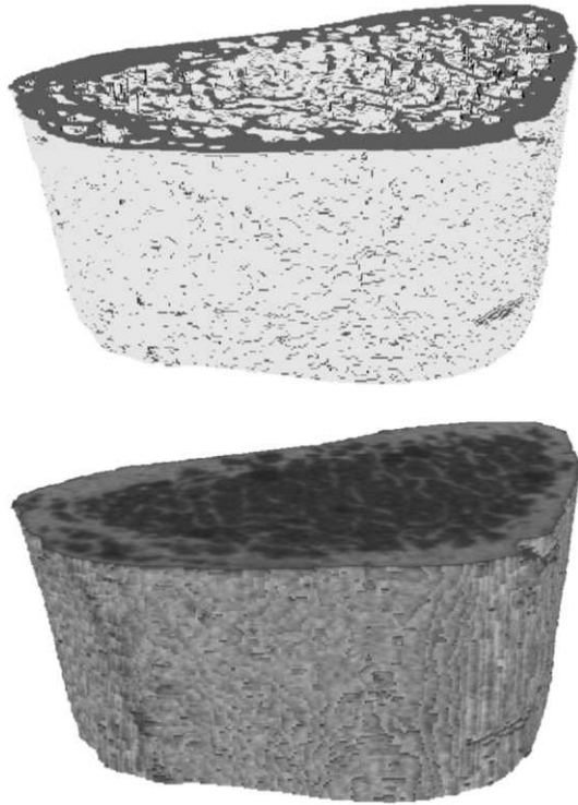
Fig. 3. Finite element voxel-based meshes of the same specimen. A typical mesh with a homogeneous tissue elastic modulus (left) and a mesh with a modulus scaled according to the CT-attenuation (right) are shown. Note that although the scaled modulus model represents the bone as a continuum, the micro-architecture is still incorporated into the model as can be clearly seen.
