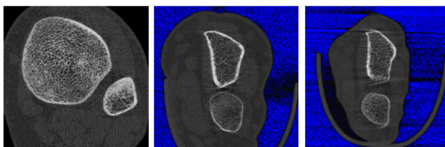
Figure 130. Example for Image Quality, good on the left, acceptable in the middle and not acceptable on the right
