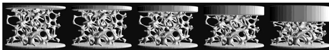
FIGURE 2 Image sequence of an aluminum foam as acquired by the image-guided failure assessment (IGFA) technique.
