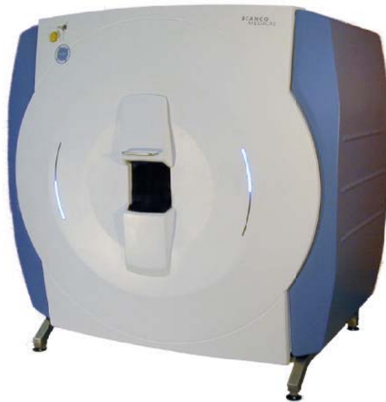
Figure 2.1: Scanco Medical XtremeCT scanner (WxDxH: 1380 x 930 x 1460 mm).
