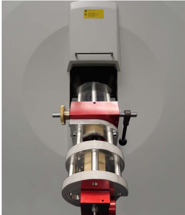
Figure 3.2: Mounted mechanical testing device in XtremeCT. The device is supported by a standard tripod (not shown in image).
