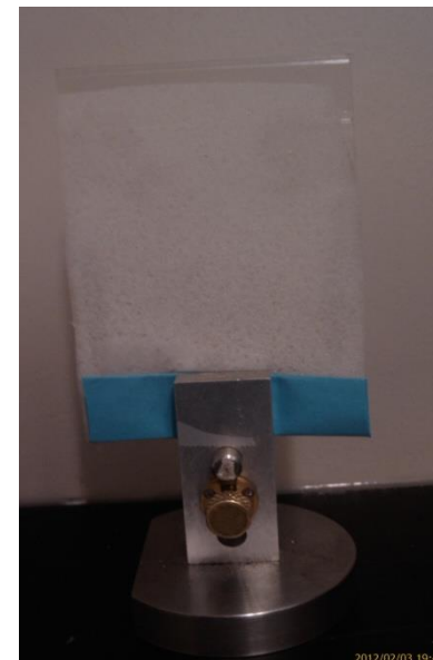
Screw clamp for large flat and/or heavier samples
