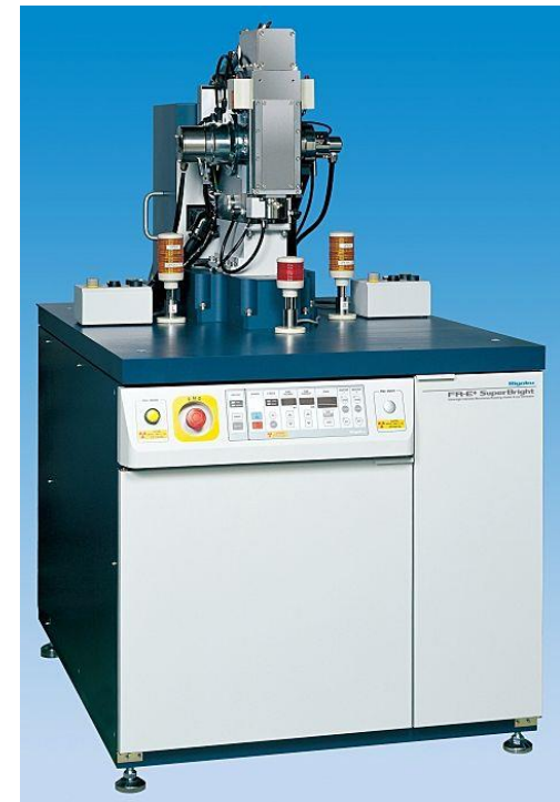
Rigaku Laboratory X-ray Source (source: directindustry.com)
