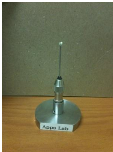
Pin vise (with Al adaptor) for small samples
