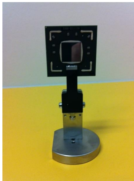
Spring clamp for medium size flat samples
