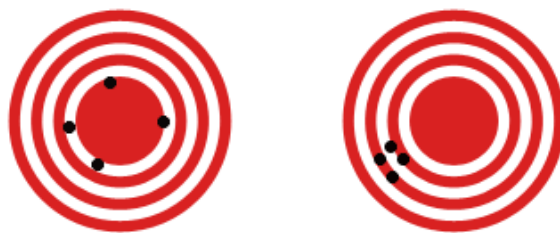
Figure 4.1: Accuracy and precision illustrated on a target. Left: High accuracy, but low precision. Right: High precision, but low accuracy.
