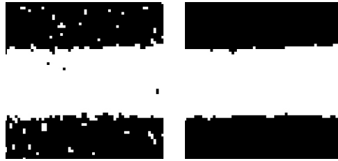
Figure 4.6: Left: Slice view of a CT scanned and thresholded drilling hole. Right: Same drilling hole, but previously erode&dilate filtered.
