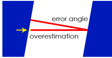
Figure 4.14: Top view on scan area. The thickness t has to be corrected by error angle \alpha .
