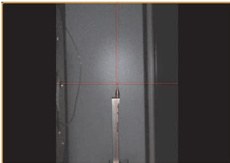
Figure 2-42 Sample Aligned with Red Crosshairs, after Adjusting Sample Y and Sample Z
