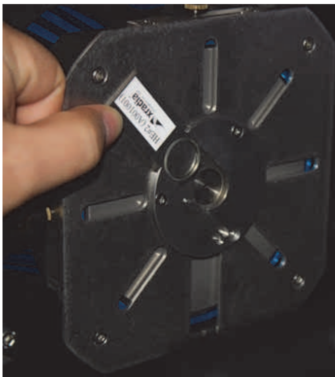
Figure F-2 X-ray Filter Installation (160 kV X-ray Source Shown)
