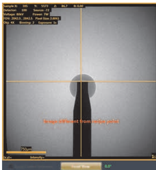
Figure 2-45 ROI Roughly Centered for Sample X and Y Axes, with Image different from recipe point Message
