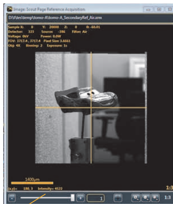
Figure 2-34 Typical Image: Scout Page Reference Acquisition Window, Displaying the Filtered Secondary Reference
