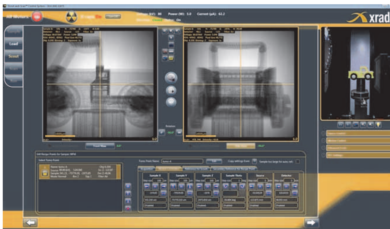
Figure 2-16 Typical Scout View – Normal Field Mode (Before Changing to Wide Field Mode)
