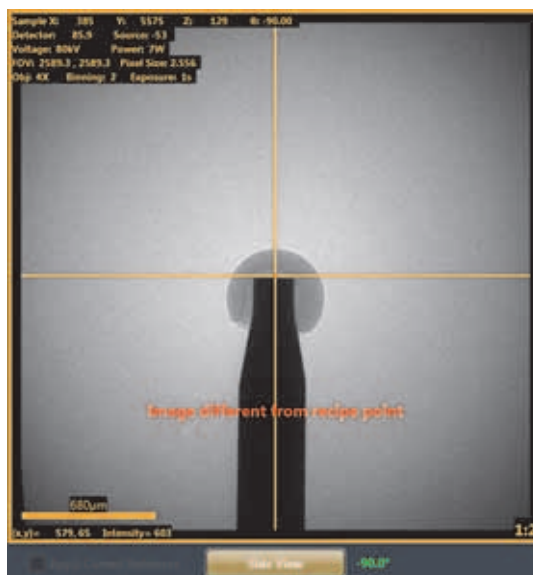
Figure 2-46 ROI Roughly Centered for Sample Z Axis, with Image different from recipe point Message
