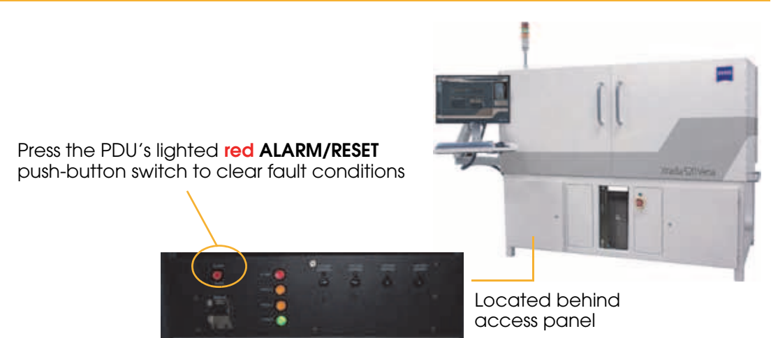
Figure A-10 Press PDU's Lighted Red ALARM/RESET Push-Button Switch to Clear Fault Conditions (Xradia 520 Versa Shown)
