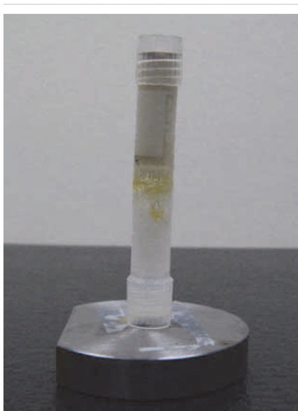
Figure E-4 Sample Holder – Sample Base with Sample in Plastic Tube
