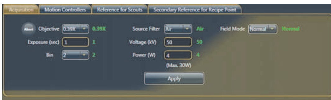
Figure 2-44 Typical Acquisition Tab within Scout View's Edit Recipe Points for Sample Panel
