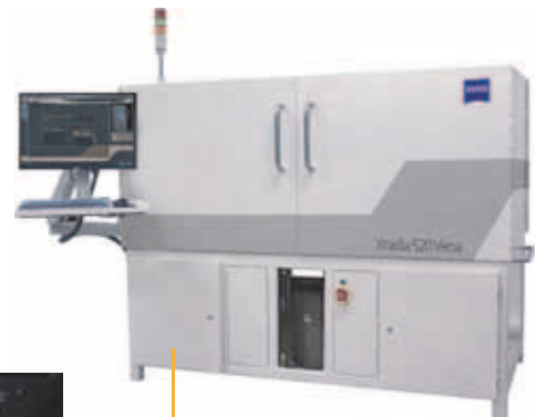
Figure A-4 Press PDU's Lighted Red ALARM/RESET Push-Button Switch to Restore X-ray Source Power (Xradia 520 Versa Shown)
