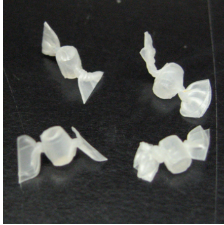
Figure 7.4: Fiducial markers wrapped tightly in Parafilm.
